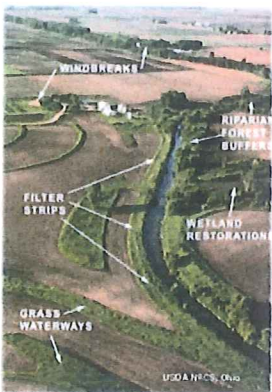
Birdseye view of an agricultural landscape with grass filter strips and other types of conservation buffer. Photo courtesy of USDA NRCS
